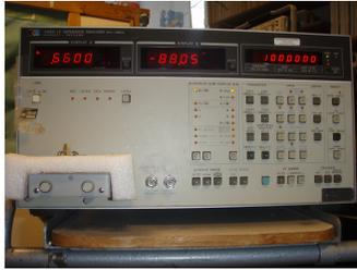
Figure 2: Impedance analyzer HP 4192A.
