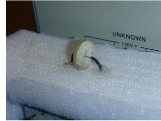
Figure 3: Piezoelectric element in measurement setup.
