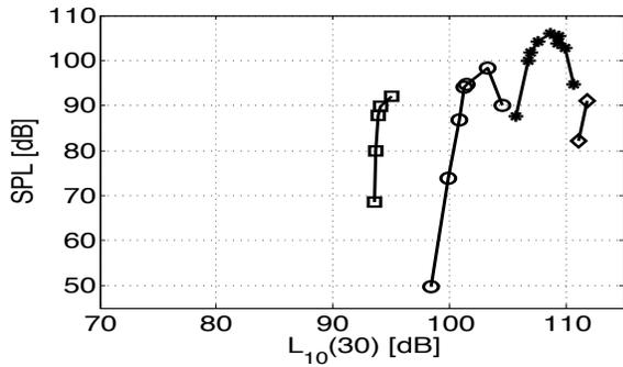
Figure 4: Resonances generated by 10 Hz tone alone. Square: 2nd mode, circle: 3rd mode, star: 4th mode, and diamond: 5th mode.
