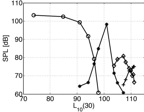
Figure 11: Effect of increasing 10Hz tone level on dominant spectrum peak. Start point is 3rd. harmonic excited with  $U_{pt} = 9.9\text{m/s}$ .
