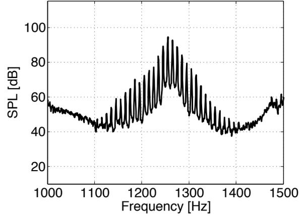
Figure 9: Close up of the resonance peak around 1250 Hz (5th longitudinal resonance) in the lower panel of Figure 8.
