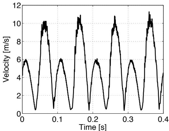
Figure 6: Hot wire measurement at center of the pipe’s entry section.  $U_{pt} = 0\text{m/s}$ ; Vacuum cleaner end closed. Loudspeaker voltage 7.5 V,  $L_{10}(30)=101.1\text{ dB}$ . Note that the hot wire used measures amplitude, not direction.
