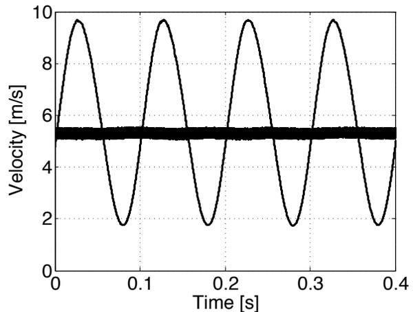
Figure 7: Hot wire measurement at center of entry section,  $U_{pt} = 10.9\text{m/s}$ . Loudspeaker voltage 9.0V.  $L_{10}(30) = 110.5\text{dB}$
