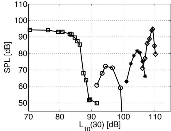
Figure 10: Effect of increasing 10Hz tone level on dominant spectrum peak. Start point is 2nd. harmonic excited with  $U_{pt} = 6.3\text{m/s}$
