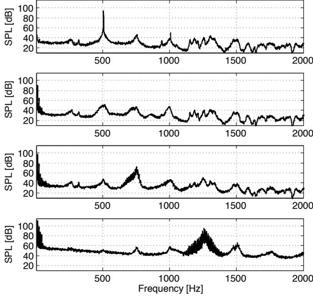
Figure 8: Influence of 10Hz tone on the second longitudinal pipe resonance. Upper Figure: resonance generated with flow velocity  $U_{pt} = 6.5\text{m/s}$  (no 10 Hz tone). Lower panels show the effect of an added 10 Hz tone at increasing levels: ( $L_{10}(30) = 0, 89.4, 96.6,$  and  $109.4$  dB)
