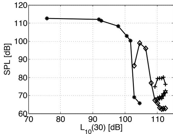
Figure 12: Effect of increasing 10Hz tone level on dominant spectrum peak. Start point is 4th harmonic excited with  $U_{pt} = 12.0\text{m/s}$ .
