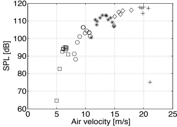
Figure 3: Sound pressure levels of dominant frequencies measured at 30mm position as function of flow velocity. Square: 2nd mode, circle: 3rd mode, star: 4th mode, diamond: 5th mode, and plus: 6th mode.
