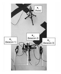
The three beacons in the lower part of the image are fixed to a frame where the baselines are all 0.59m. The host is located at a variable distance away from the beacon network. Shown here the host is approximately 2m from the beacons.
