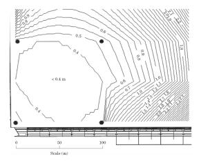
Plan view of the dam and hydrophone locations showing a contour plot of position errors for a depth of z = 49m.
