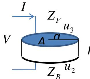
Fig.1. The parameters of piezoelectric circular disc as used in modelling of impedance frequency response for thickness mode of vibrations.
