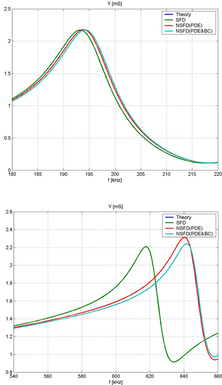
*Fig 2. The admittance frequency response of 200kHz piezoelectric disc in thickness mode of vibration for first (upper chart) and second (lower chart) mode as obtained with analytical and discrete methods. For comparison purposes the discrete solutions are presented for standard scheme, nonstandard scheme applied in PDE only and nonstandard scheme in PDE and in boundary condition.*
